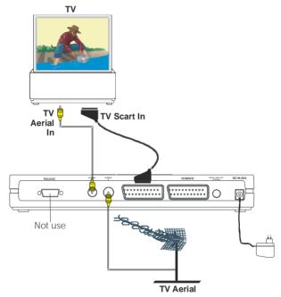
If you have a VCR or other equipment connected to your television, please connect the receiver as described here and refer the "Connecting the external devices" on page 19.
